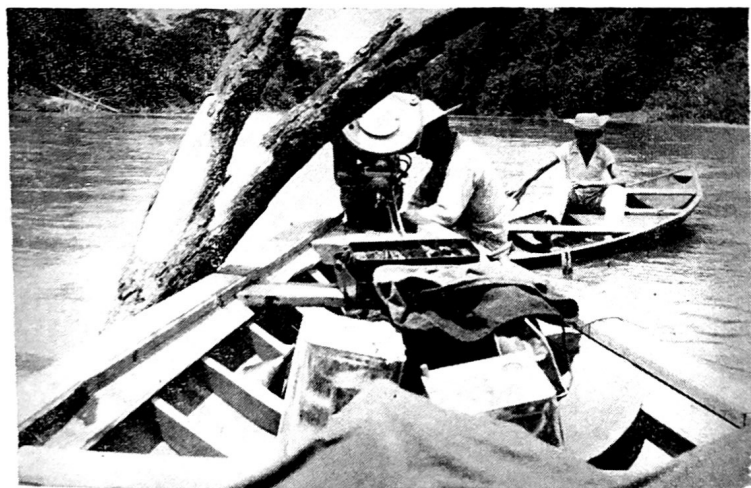
Putting in a new pin in the propeller of the outboard motor in one of the rivers in the Acre Territory, while John Hatcher was on a journey there. Many trees and limbs are in the streams and when the propeller strikes one it shears a pin. This happens often while on a journey. John Hatcher is in the front of the boat taking the picture.
